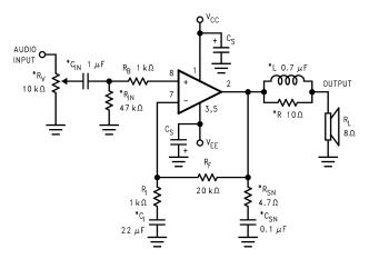
Figure 4. Auxillary Amplifier Application Circuit
