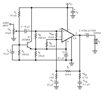
Figure 3. Single Supply Amplifier Application Circuit
