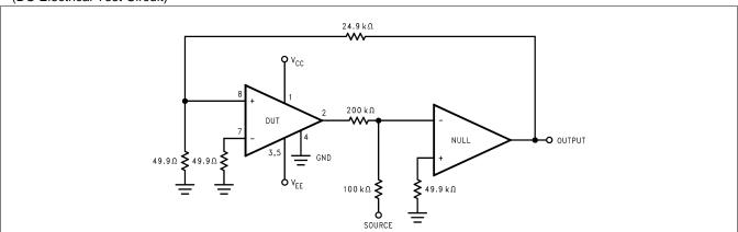
(1) DC Electrical Test; Refer to Test Circuit #1.
