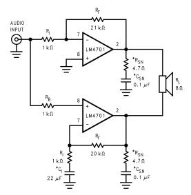
Figure 2. Bridged Amplifier Application Circuit
