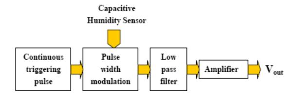
This sensor support electronic circuitry uses two timers. One timer continuously issues a pulse train in order to trigger the other timer, which operates in PWM mode.
